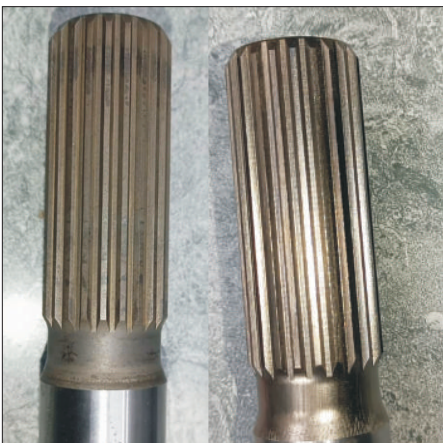
Before (Rust) After
